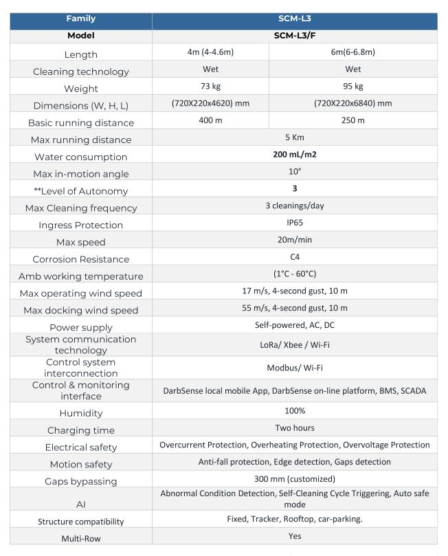
\*W/D: REFERS TO WET CLEANING TECHNOLOGY/ DRY CLEANING TECHNOLOGY \*\*LEVEL OF AUTONOMY: LEVEL "]" REFERS TO PORTABLE LEVEL "2" REFERS TO WITH OPERATOR LEVEL "3" REFERS TO NO OPERATOR
